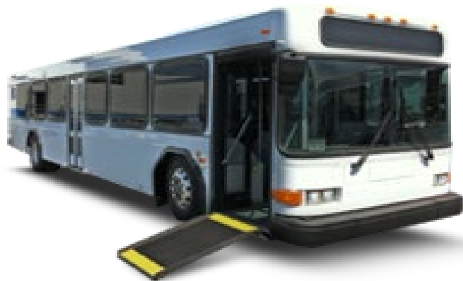
Figure 6-17: Low Floor Heavy Duty Bus
